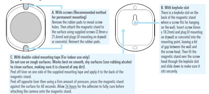
**IMPORTANT:** Ensure that the surface and fixing points are strong enough to sustain the weight of the camera and magnetic stand.
