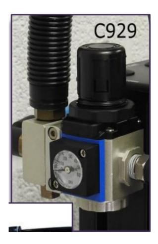
An LPR is a nice option to have because it allows the operator to adjust the down force of the ram cylinder independently from the driver head main regulator. This is particularly useful on more sensitive applications such as fine thread bottles, serrated driver applications and 4 lug steel caps.
