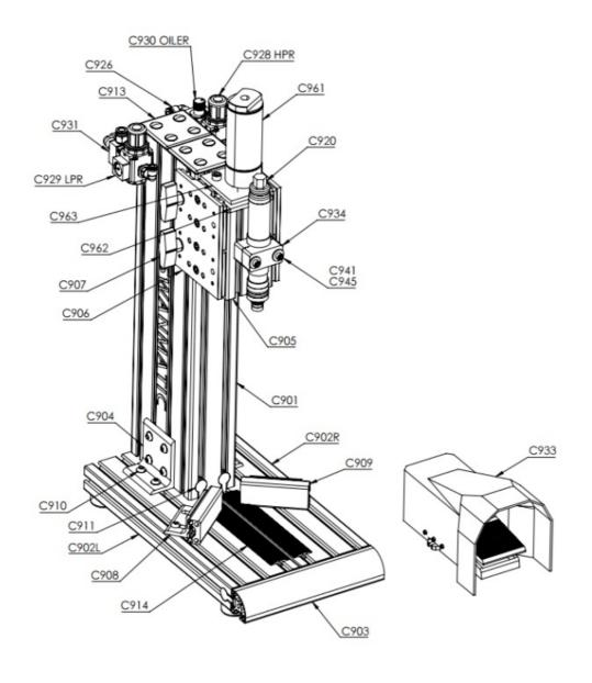
Taller Columns and Driver Spacer Blocks can be Ordered for Larger Bottles C900 Parts Call Out
