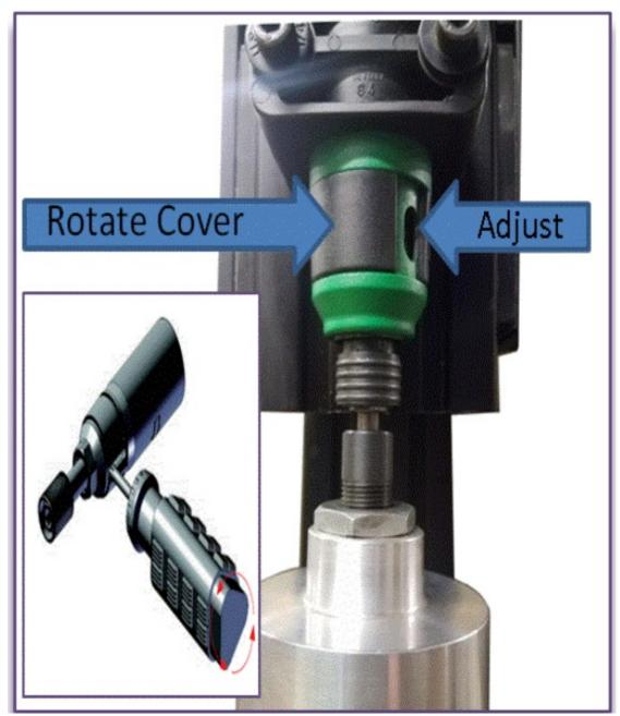
**NOTE:** The capper will not engage until a bottle is actually placed in the capper and the driver shell comes in contact with the cap. When the drive shell comes in contact with cap it will triggers the driver to rotate.
