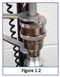
Accurate alignment of the container cap to the insert and proper height and torque settings are critical for optimum capping results. Rotate the spindle until it reaches the bottom of its stroke.
