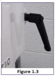
Place an already capped container under the insert, adjusting the capper height so that the container cap just contacts the insert. The height of the capper head is adjusted by loosening the column locking handle (Figure 1.3) and rotating the adjustment handle (Figure 1.4).
