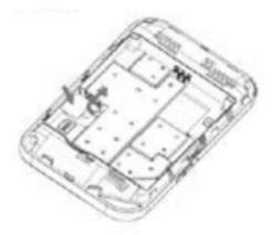
3. Insert the Battery and attach the battery cover
