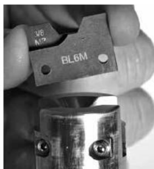
Fig. 6 Removing the coning blade
