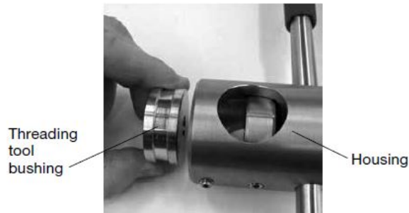
Fig. 13 Removing the threading tool bushing
