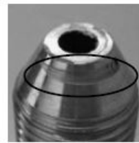
Non-conforming Severe tearing on cone
