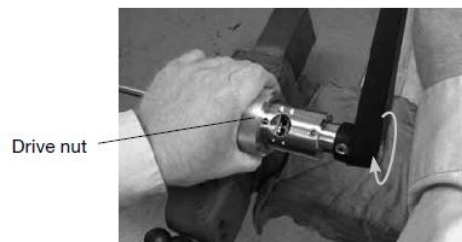
Fig. 24 Turning the handle and advancing the drive nut
