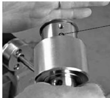
Fig. 18 Exposing the end of the coning tool
