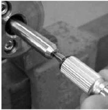
Fig. 37 Deburr the tube ID
