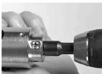
Fig. 31 Inserting the power adapter into drill chuck
