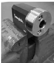
Fig. 32 Placing the tube vise in a bench vise
