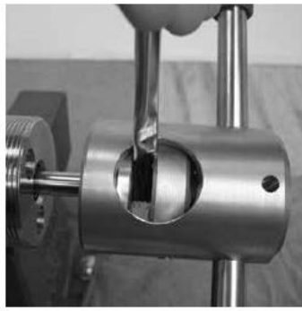
Fig. 41 Removing the threading tool and chips
