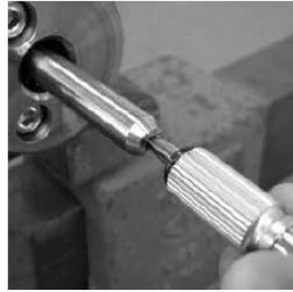
Fig. 26 Deburr the tube ID
