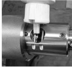
Fig. 23 Applying cutting fluid through the chip window
