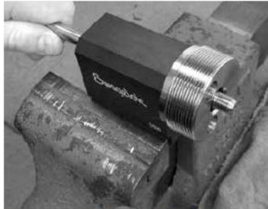
Fig. 42 Removing coned/threaded tube from vise
