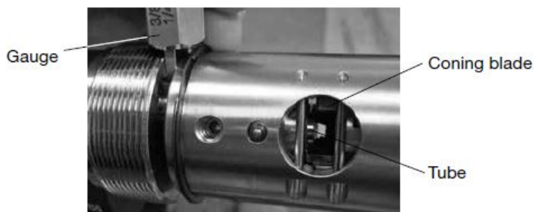
Fig. 34 Verifying the tube is in contact with coning blade
