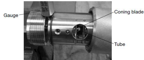
Fig. 20 Verifying the tube is in contact with coning blade
