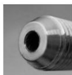
Acceptable ID of the nipple properly deburred.
