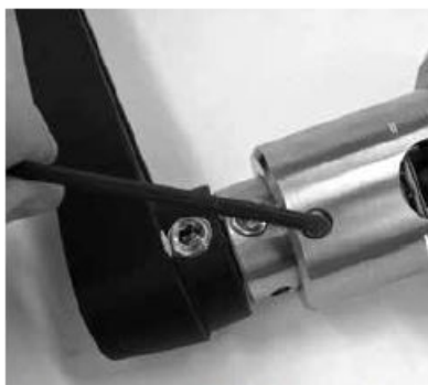
Fig. 3 Loosening the 1/4 in. set screw (second screw is on opposite side of housing)
