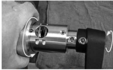
Fig. 25 Loosening the drive nut
