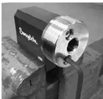
Fig. 2 Removing/Attaching the manual adapter
