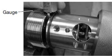
Fig. 19 Using the coning gauge to establish the gap
