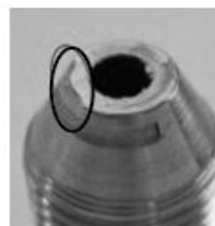
Non-conforming damaged cone face diameter dropped. Note the tearing on the cone, face, and ID of the nipple has not been deburred.
