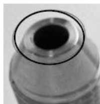
Acceptable uniform appearance of radius around cone face diameter.
