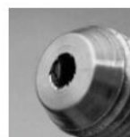
Non-conforming burrs present in ID of the nipple. Note: Image shows a cone ID that has not been deburred and tearing is shown on the cone.
