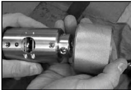
Fig. 29 Removing the drive nut
