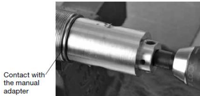
Fig. 36 Advancing the coning tool
