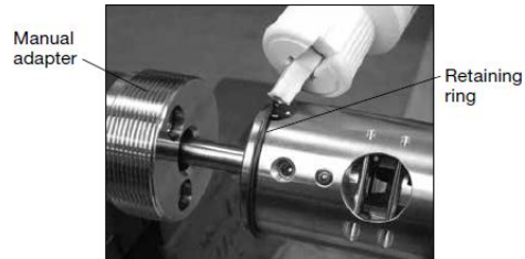
Fig. 21 Applying cutting fluid to retaining ring
