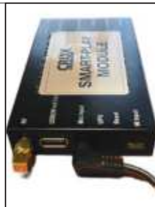
12. Plug in the microphone cable to the Smart-Play module. Optional plug in original smartphone cable to USB Ext. cable for wired connectivity
