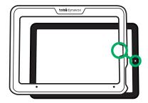
3 Press the iPad/plate assembly into the Speech Case Mini body.
