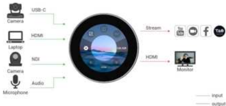
TAO 1mini-HN SYSTEM CONNECTION DIAGRAM
