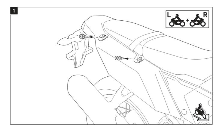
**NOTE:** When mounting the luggage rack with the SW-MOTECH side carrier, the screws (3) are not required. Mount instead the marked /•J parts of the side carrier and the spacers (6), as shown in the drawing. Insert the plastic plugs (2) into the mounting struts (1). Attach the mounting struts (1) to the vehicle, as shown in the drawing. ATTENTION: Use liquid thread locker! Do not fully tighten the screws yet.
