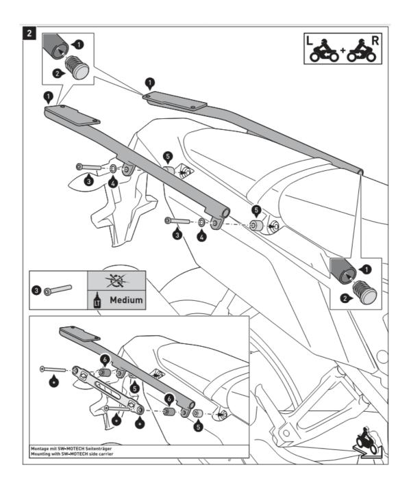
**NOTE:** Choose the marked front mounting position (Al or the rear mounting position (BJ of the luggage rack according to your preferences, as shown in the detail drawing. Attach the luggage rack (7) to the mounting struts (1 I. as shown in the drawing. Once all parts are evenly positioned without excess tension, tighten the screws (8) as specified. Tighten the screws (3) (see step [211 with the manufacturers' specified torque
