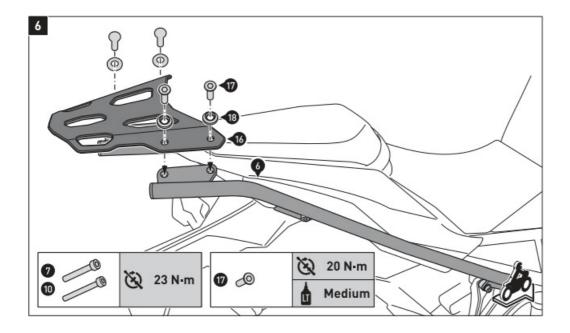
Attach the luggage rack (16) on both sides to the mounting struts (6), as shown in the drawing.
