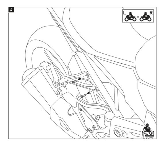
Loosen the screws of the passenger footrest mount, as shown in the drawing.
