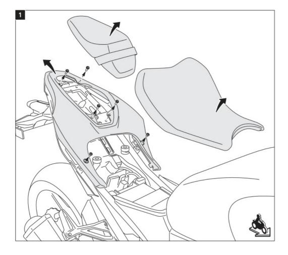
Remove the seat and the screws from the vehicle, as shown in the drawing. Take the rear panel off, by pulling it to the rear.
