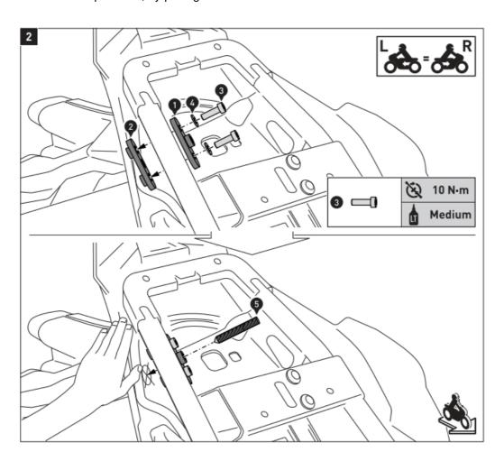
Attach the mounting bracket (1) and the counter bracket (2) to the opening in the rear frame, as shown in the drawing.
