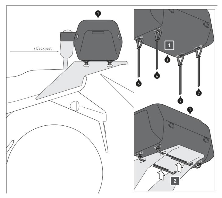
**ATTENTION:** All components of the tail bag must not contact any hot or moving parts of the vehicle. All parts should also remain 5 cm away from hot parts of the vehicle and remain clear of the exhaust stream.
