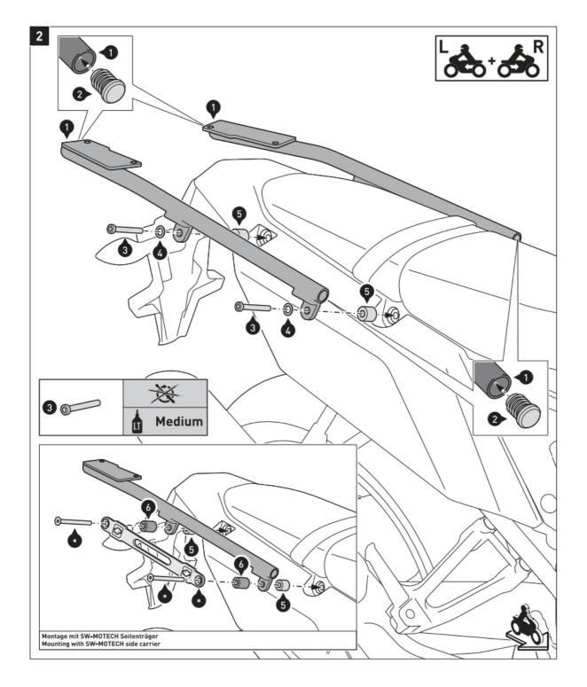
**NOTE:** When mounting the luggage rack with the SW-MOTECH side earner, the screws /3) are not required. Mount instead the marked parts of the side carrier and the spacers [6)], as shown in the drawing. Insert the plastic plugs [2) into the mounting struts (1).
