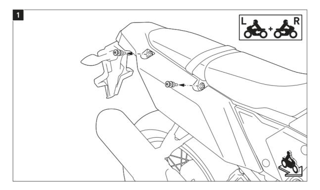
**NOTE.** The mounting is shown on the right side of the vehicle only. Repeat the same procedure on the left side of the vehicle with the appropriate parts.
