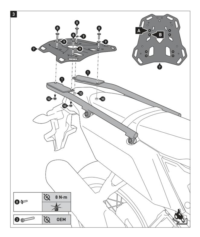
**NOTE:** Choose the marked front mounting position (A) or the rear mounting position [BJ of the luggage rack according to your preferences, as shown in the detail drawing.
