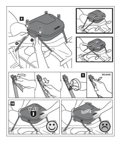
**Step [8]:** Attach the hook buckles of the loop straps [11 I on both sides to the marked loops of the top case [1 I. as shown in the drawing. Tighten all loop straps until the top case [1) is centered and securely fastened to the vehicle.
