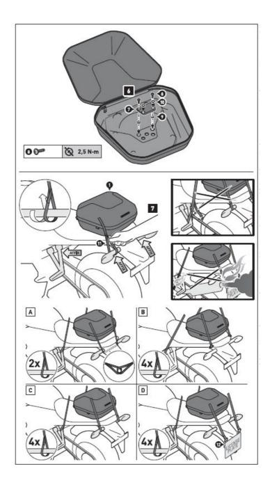
Step [6]: Attach the cover plate (7) inside the top case (11. Tighten the screws as specified in the parts list.
