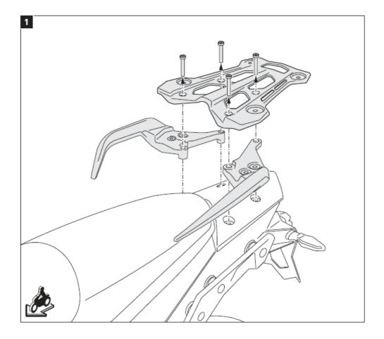
**NOTICE:** Use for mounting to the Duke 790 Adventure the screws (7) and (BJ instead of the screws (2) and (5). Attach the mounting brackets (1) with the passenger grips to the vehicle.
