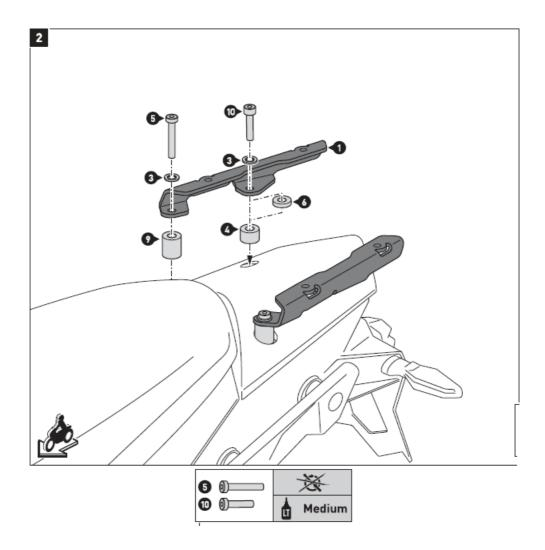
**NOTICE:** Choose the marked front or rear mounting position {A I BJ according to your preferences. If necessary remove the seat while mounting the luggage rack {11J.
