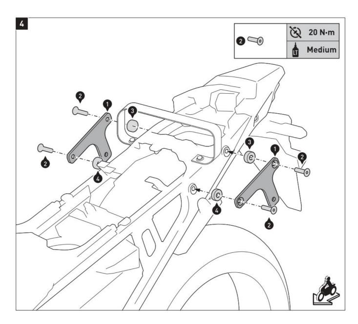
Attach the mounting brackets (1) on both sides to the vehicle, as shown in the drawing.
