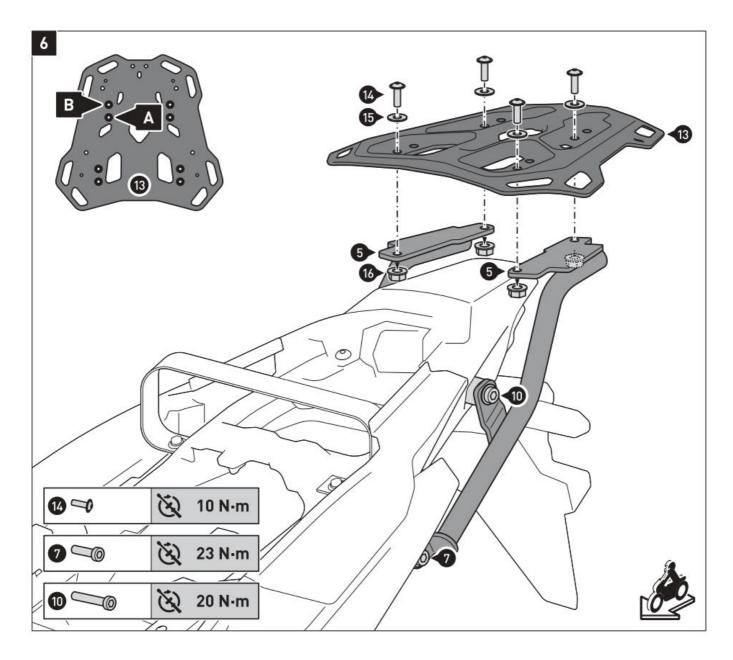
NOTE: Depending on the available space, attach the luggage rack to the marked mounting position (A) or (B), as shown in the detail drawing. Attach the luggage rack (13) to the mounting struts (5). as shown in the drawing.
