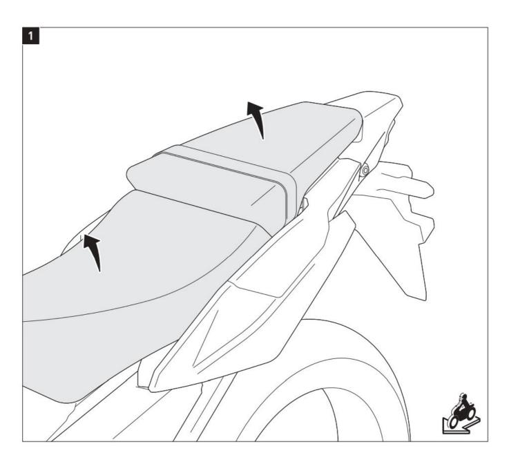
Remove the seat bench and the passenger seat from the vehicle.
