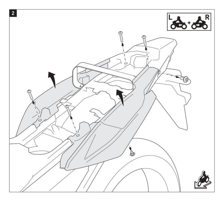
Remove on both sides of the vehicle the shown screws and then the rear side fairings from the vehicle. Pay attention to the plastic hooks of the side fairings.
