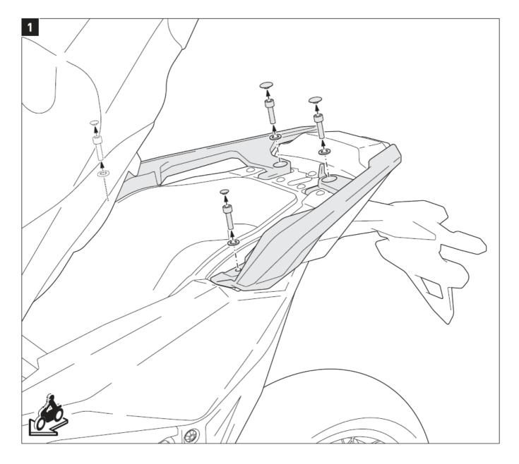
Insert the plastic plugs (2] into the ends of the mounting struts (1), as shown in the detail drawing. Attach the mounting struts (1) to the vehicle, as shown in the drawing.
