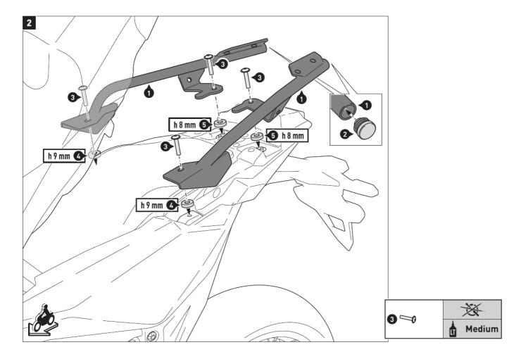
Attach the luggage rack (6) onto the mounting struts (1), as shown in the drawing.
