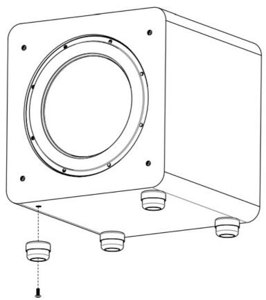
**Important Notice**: When placing the subwoofer back into position, do not allow the weight of the cabinet to place an excessive lateral (sideways) load on the Isolation feet. This may damage the Isolation feet, the threaded insert or the cabinet.
