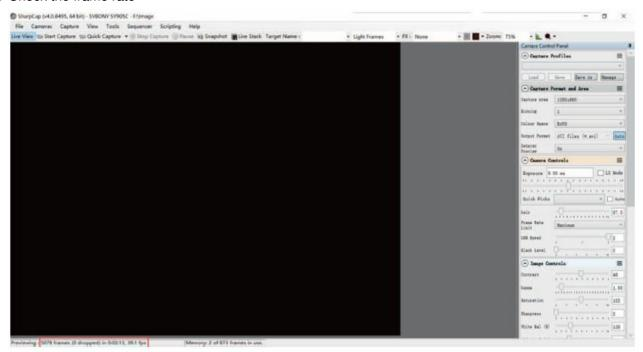
2. Remove the camera dust cover and adjust the exposure time; There are light and dark changes in the preview interface, indicating that it is working properly.
