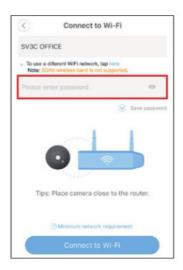
If it fails to connect. please reset and power off the camera to try again. WIFI name and password should not contain any special characters such as "% # \$ @\_±.. and blank. WiFi password should be within 8-19 characters
