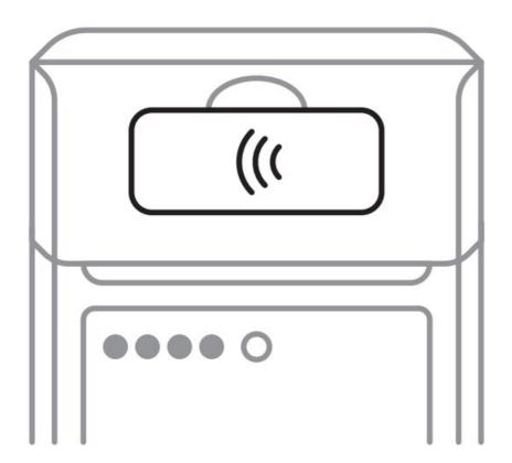
Note: The IC card reader is can be easily stained with dirt after prolonged use of the POS. Please use a proper clean napkin to clean the dirt.
