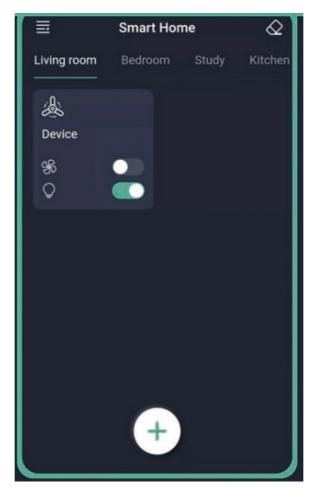
Unpair button. Click this button within 5 seconds when the device is powered on, If the device flashes or beeps, it means that the phone is unpaired with the device and the phone will not be able to control the device when in the room page, long press the device card you can delete the device or change the device name.
