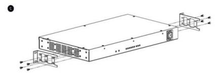
C Option-Mounting Ear Mount Bracket at the Center Secure Ear Mount Brackets to the Unit using eight Flat head screws
