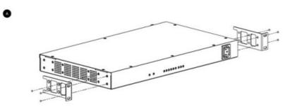
A Option-Mounting Ear Mount Bracket at Front Secure Ear Mount Brackets to the Unit using eight Flat head screws
