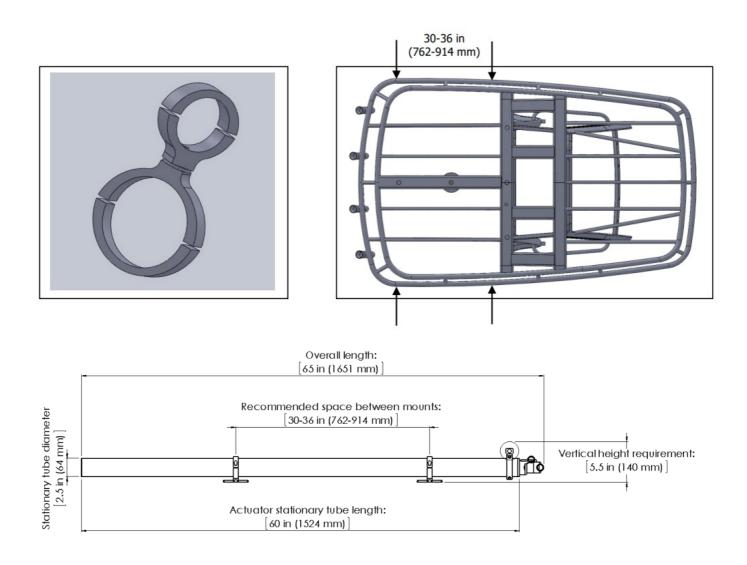
**STEP** 2: DETERMINE SHADE WIDTH. MTF framework (stationary actuator) and mounting clamps an obstruction-free area shown below.
