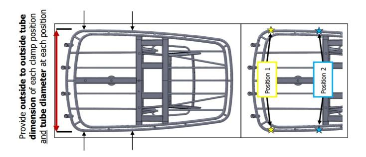
MTF shade width is specified by the "outside to outside" tube dimension – outside of PORT actuator to outside of STBD actuator. The maximum possible width for an MTF shade is 96"
