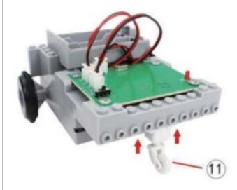
Attach the eyes 4 to the eye base 13, and the eye base to the T-block 5. Then attach them to the circuit board mount 12.
