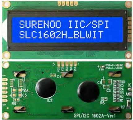
The SLC1602H Series LCD Module is a product manufactured by Shenzhen Surenoo Technology Co., Ltd. This module is designed to display characters and is compatible with the AIP31068 Reference Controller Datasheet.
