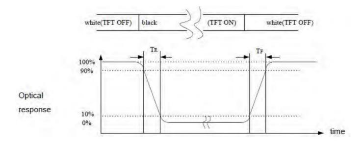
Note 4: Definition of optical measurement setup
