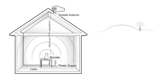
Before installation, ensure there will be adequate separation between the planned locations of the outside antenna and booster (at least 25 ft.).
