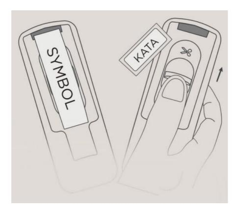
After inserting or replacing a new roll of label, click the printer's power button to print a blank label to let the print head identify the label position.
