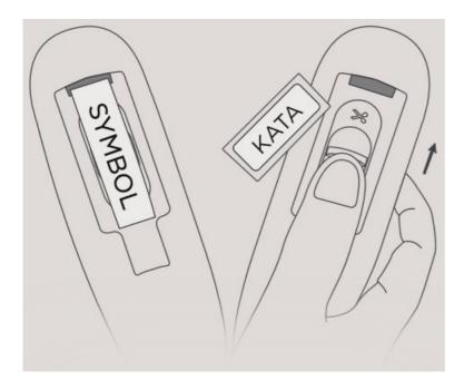
After inserting or replacing a new roll of label, click the printer's power button to print a blank label to let the print head identify the label position.
