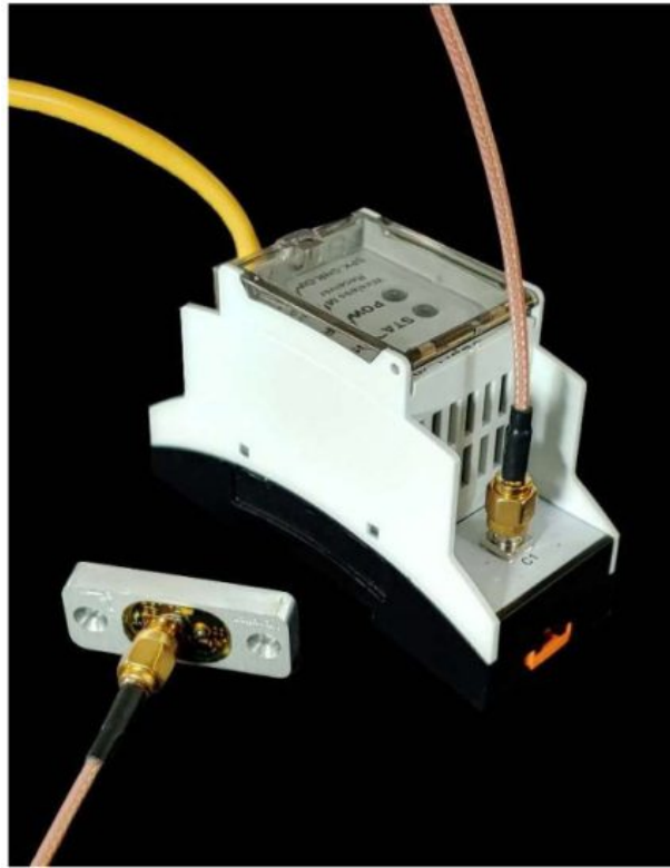
Figure 2 Example coax vibration sensor connected to WMR in wired configuration; both power and data to and from a sensor are transmitted via a single SMA coaxial connection.
