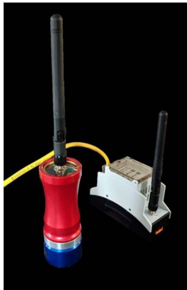
Figure 2 Example coax vibration sensor connected to WMR in wired configuration; both power and data to and from a sensor are transmitted via a single SMA coaxial connection.
