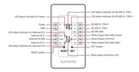
• Press INIT button to reset Secure I/O 2 interworking with a device and then connect to another device.
