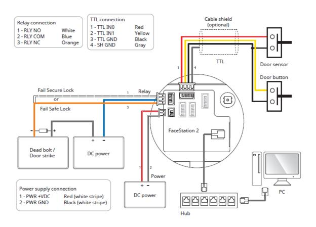
• Suprema's standalone intelligent readers contain internal relays that can directly lock/unlock doors without external controllers for added convenience. For access control applications in need of security, however, it is NOT recommended to use the internal relay of a reader to prevent any tampering attacks that can potentially
