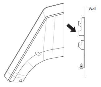
• Connect FaceStation 2 to the bracket by rotating the product fixing screw of FaceStation 2.
