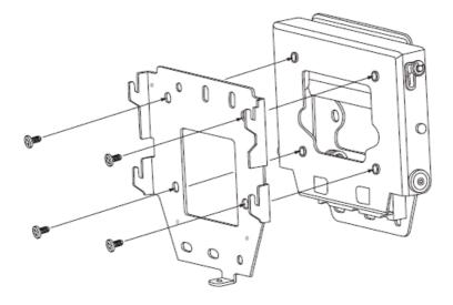
• Install FaceStation 2 onto the fixed bracket.
