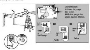
5 Within 30 seconds, press and hold the programmed button of remote until garage door opener lights flash or two clicks are heard it has learned the code.
