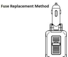
Pull out the damaged fuse from the bottom of the machine and insert the spare fuse inside the box into the hole to resume normal use
