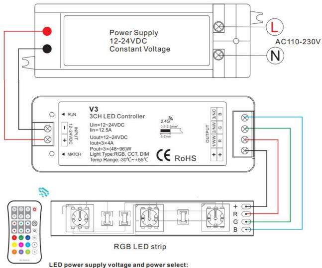
12V lamp, Input 12V power supply, can load 0~144W,
