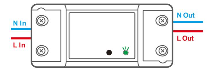
The device will exit the quick pairing mode if not paired within 3mins. If you want to enter this mode, please long press the manual button for about Ss until the Wi-Fi LED indicator changes in a cycle of two short and one long flash and release.
