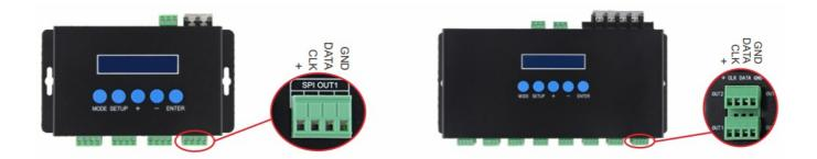
To output LPD6803/LPD8806/P9813/WS2801 controlling signal, it required at least three lines:
