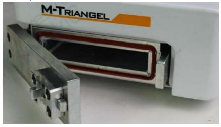
Press the start button, about 30 seconds, you can press the stop button, take out the screen.
