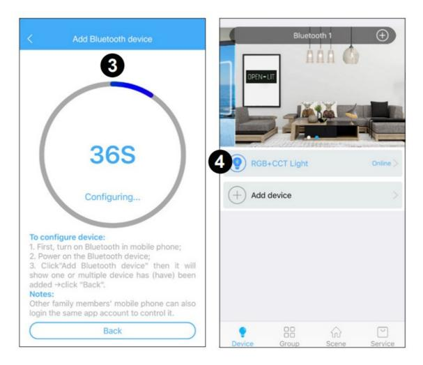
**Note:** Each time the mode on the dimmer is changed, the dimmer will need to be re-paired with account on phone/tablet.
