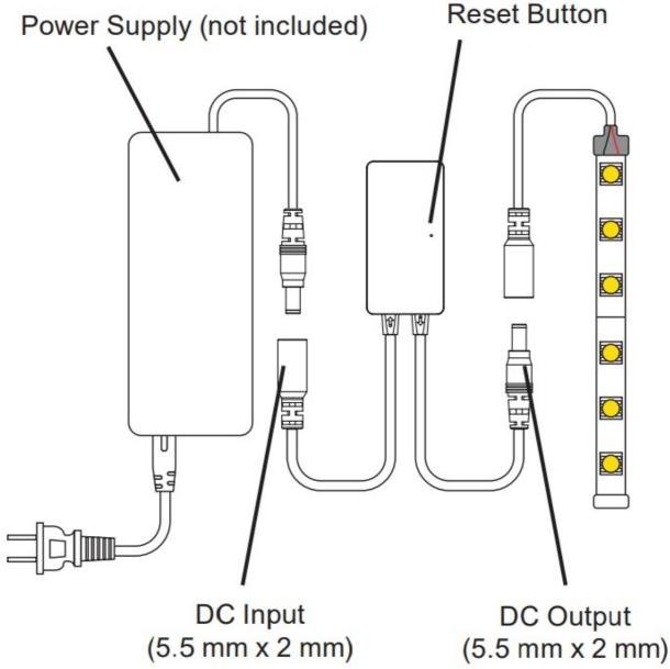
The reset button can be used to unpair dimmer. If dimmer has issues pairing, this can also be used to reset to default settings.
