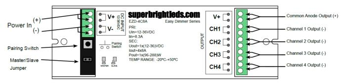
CH1 and CH3 are Warm White Channels CH2 and CH4 are Cool White Channels
