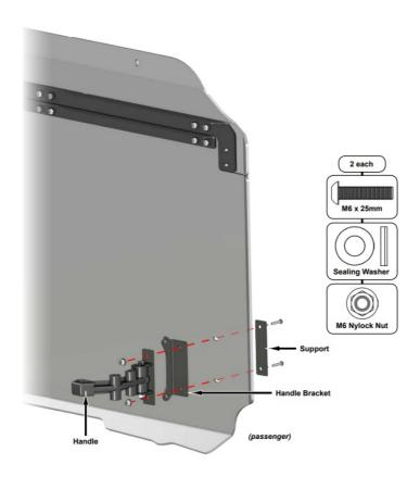
• Place the Windshield in the open position and secure the Struts to Handle Brackets and Upper Brackets with hardware is shown; tighten hardware
