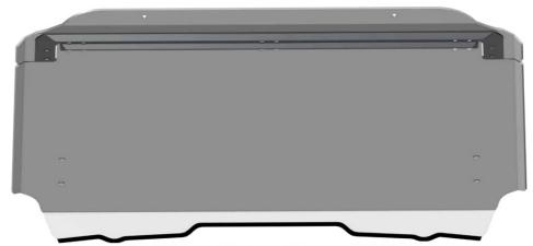
Install Seal along lower edge of Windshield as shown.
