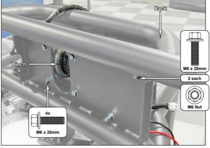
• Install Winch and Box to Rack with hardware shown; tighten.
