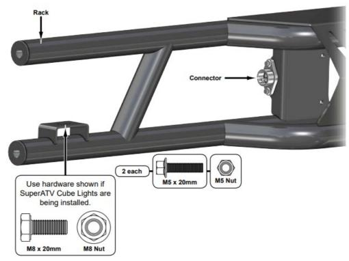
• Install Rack to Right and Left with hardware and components shown; tighten.
