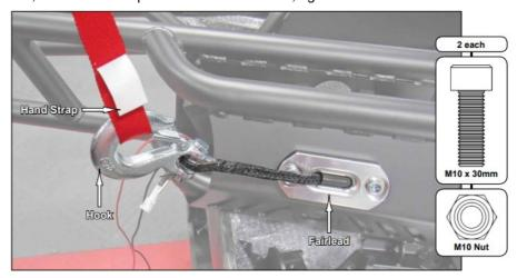
• Install Connector to Rack with hardware shown; tighten.
