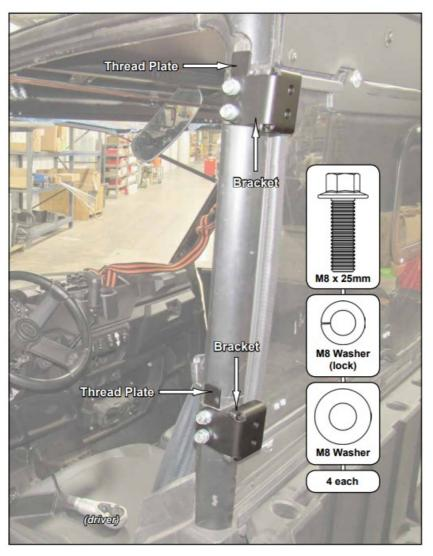
If SuperATV Cab Enclosure Doors are not installed, use Bolt size shown.
