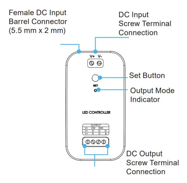
The output mode indicator will be GREEN when in single color dimming mode, BLUE when in CCT mode, and RED when in RGB mode.
