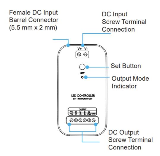
The output mode indicator will be GREEN when in RGBW mode and BLUE when in RGB+CCT mode. To switch between modes, simply hold the set button until output mode indicator changes color.
