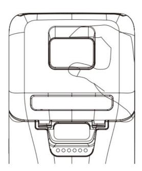
**Step 2:** Put paper in the bin, and notice the position and direction of the paper and keep part of the paper outside the bin
