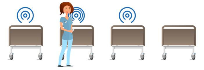
In pairing mode, the light/sound frequency will increase when the HB200 gets closer to a control box.
