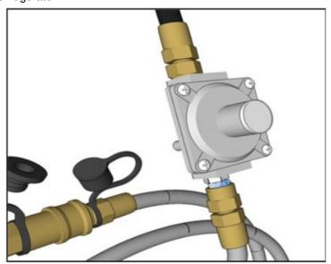
Test connection from gas line to adapter
