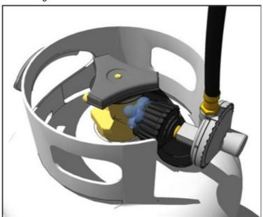
Test connection from burner to LP Hose
