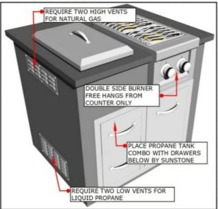
**WARNING:** Never build shelf or enclose interior space under the Burner Cut-Out. The Side Burner is Self-Rimming and is supported by the top counter. The bottom of Burner needs to be open to allow for proper ventilation. ALLOW 6 INCH MINIMUM CLEARANCE FROM UNDERSIDE OF COUNTER BURNER BACK TO INTERIOR ISLAND WALL – MUST ALLOW AIR FLOW AROUND BACK OF BURNER.
