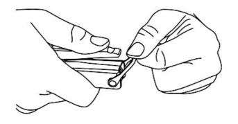
To use the Pliers, squeeze the handle firmly to release the tail lock. Always make sure the tail lock is fully engaged before using the other tools.
