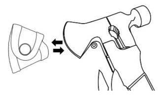
Axe blade cover for safety. Carefully remove blade guard before use, replace when done to protect the blade.
