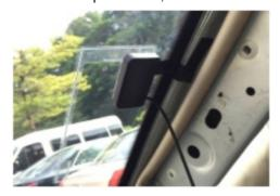
3. Ensure antenna Ground(black) contact to metal car body well
