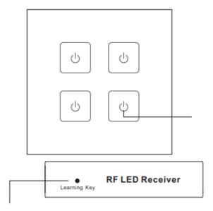
• Step 1:Do wiring the wall panel & RF receiver according to the wiring diagram (please refer to the instructions
