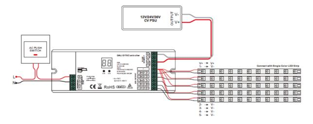
Note all 5 channels are controlled together under this mode.
