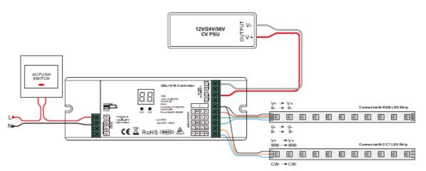
Note brightness of both RGB & CCT LEDs can be controlled, color control only applicable to RGB LED under this mode.
