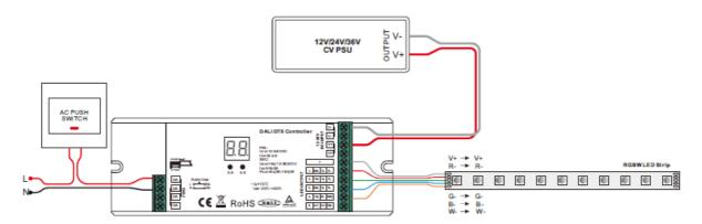
Note only the RGB LED can be controlled under this mode.
