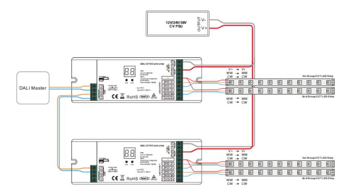
Please make sure that the DALI master controller supports Tc color type commands. The control gear will be discovered by master controller as 2 separate Tc devices.
