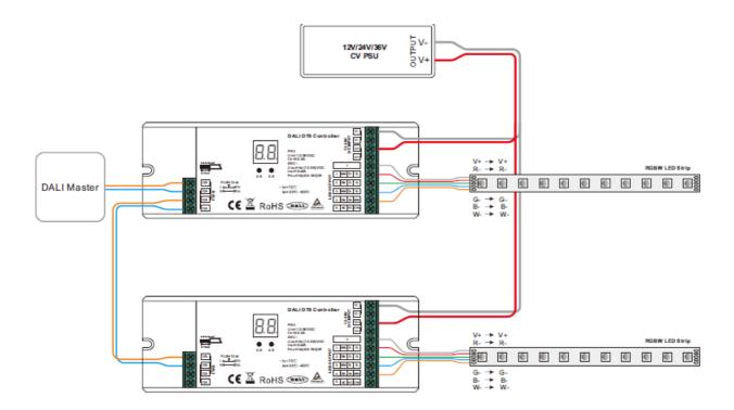
Make sure that the DALI master controller supports RGBWAF & Tc color type commands. The control gear will be discovered by master controller as 2 separate devices: RGB, Tc.
